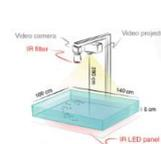
**Fig. 1 Experimental setup.** Groups of fish of around 50 individuals were filmed in a large and shallow tank, while the ambient illumination is continuously modified over time using a video projector. The video system is built using a custom built infrared LED panel, and the movements of the fish are recorded using an overhead camera through one of the 48 x 48 camera eye lenses that make up the camera. In order to avoid that the variations alter the lighting conditions of the tank.
